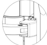
2. Insert the damper adjuster. Push in all the way.
