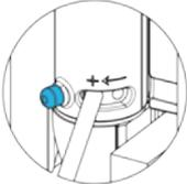
2. Apply pressure in the + direction on the speed tool until you can remove the speed pin. Then allow the tool to rotate to the base of the arrow to reduce speed.
