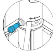
3. Insert the speed pin all the way back in, release the pressure of the speed tool and remove it.
