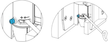
2. Apply pressure on the speed tool in the + symlbe direction until you can remove the speed pin. Then push the tool to the + symlbe to increase speed.
