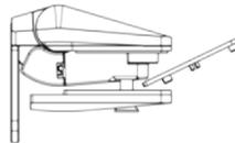
5. Pre drilling the holes for harder timbers or masonry. Then secure the first 2 wall screws on the top hinge into the timber. Repeat for the lower hinge. carefully open the gate and secure the other 2 screws on each hinge.
