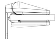
6. Push packers in above the hinge for the glass to rest on. They should be pushed in past the level of the glass (see diagram). Repeat step 6 for bottom hinge.
