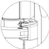
1. Open the gate and slide out the damper adjuster.
