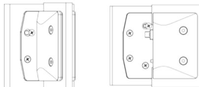
3. Take one hinge and slide it into the gate panel. With the hinge in the center of the cutout push all the way to the back of the cutout tighten the cover plate screws. Repeat these steps for the lower hinge.
